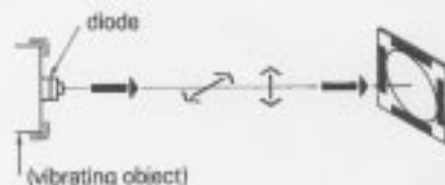
Analyze Target Vibration and Deflection. Use a collimated laser diode or LED attached to the target under investigation to optically generate position information at the PSD
